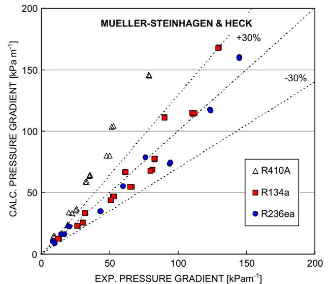
Fig. 16. Calculated vs experimental pressure gradient: the Mueller-Steinhagen and Heck correlation.
