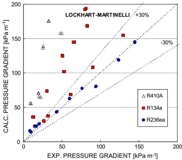
Fig. 9. Calculated vs experimental pressure gradient: the Lockhart and Martinelli correlation.
