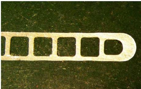
Fig. 1. Enlarged image of the multiport minichannels test tube.
