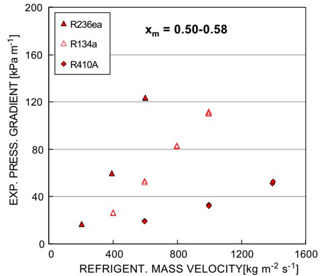
Fig. 8. Experimental frictional pressure gradient vs mass velocity at constant vapour quality for the three refrigerants.
