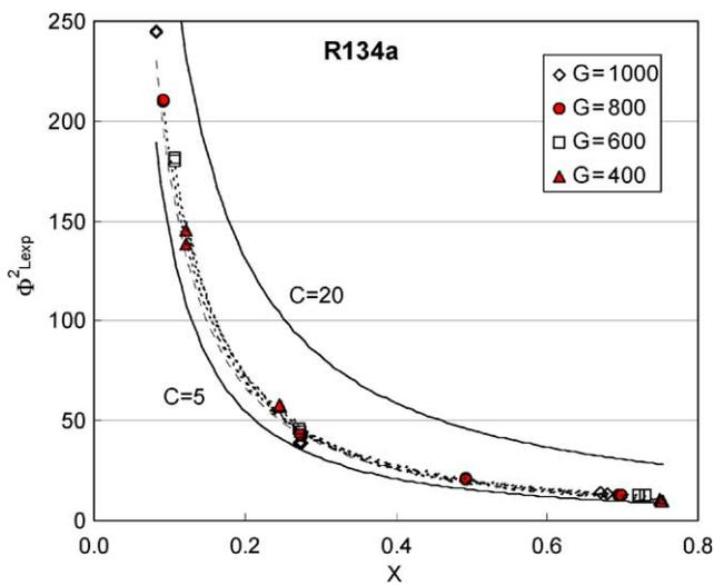
Fig. 10. R134a experimental two-phase multiplier vs Martinelli parameter.
