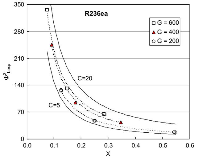
Fig. 11. R236ea experimental two-phase multiplier vs Martinelli parameter.
