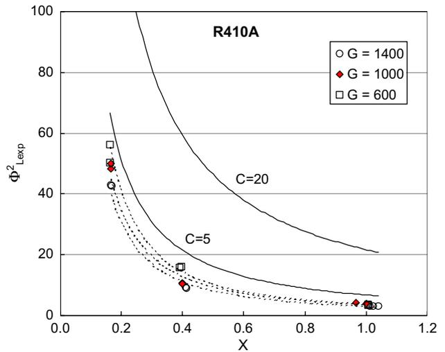
Fig. 12. R410A experimental two-phase multiplier vs Martinelli parameter.
