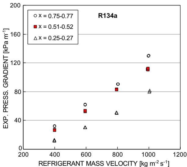
Fig. 4. R134a experimental frictional pressure gradient vs mass velocity.
