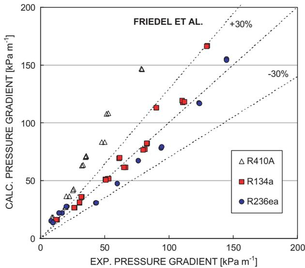
Fig. 13. Calculated vs experimental pressure gradient: the Friedel et al. correlation.
