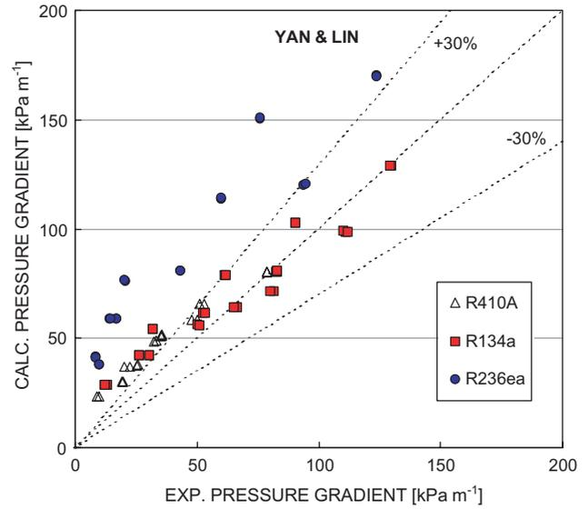
Fig. 19. Calculated vs experimental pressure gradient: the Yan and Lin correlation.
