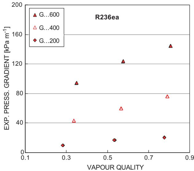
Fig. 6. R236ea experimental frictional pressure gradient vs vapour quality.
