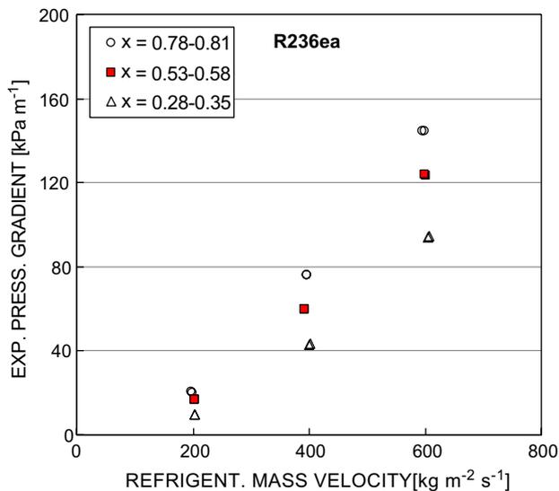
Fig. 7. R236ea experimental frictional pressure gradient vs mass velocity.
