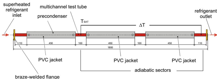
Fig. 3. Experimental test section (measures in millimeters).
