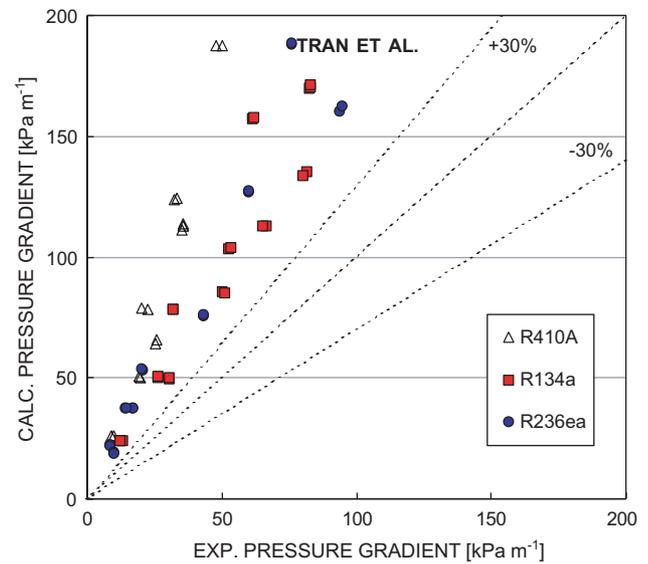
Fig. 15. Calculated vs experimental pressure gradient: the Tran et al. correlation.
