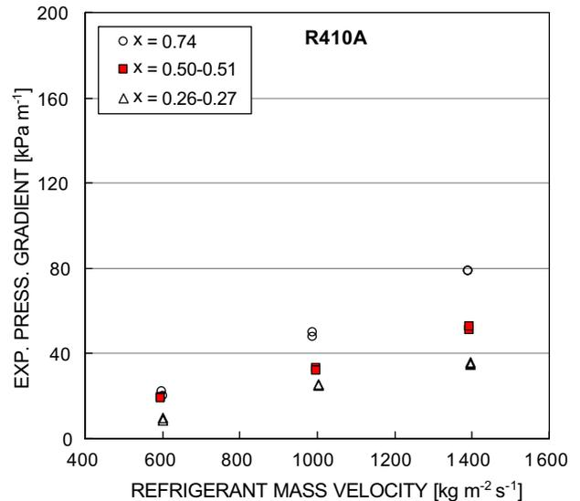
Fig. 5. R410A experimental frictional pressure gradient vs mass velocity.
