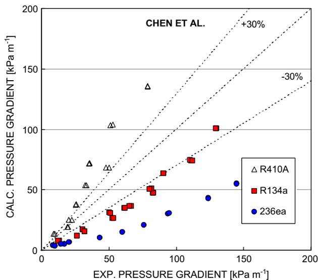
Fig. 14. Calculated vs experimental pressure gradient: the Chen et al. correlation.
