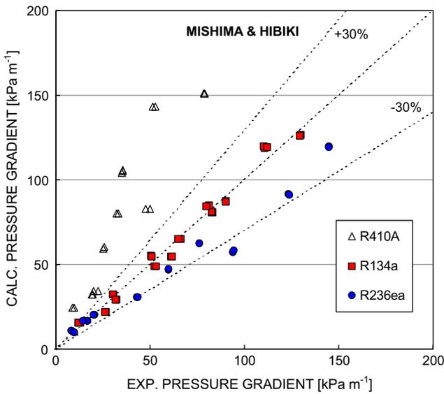
Fig. 18. Calculated vs experimental pressure gradient: the Mishima and Hibiki correlation.
