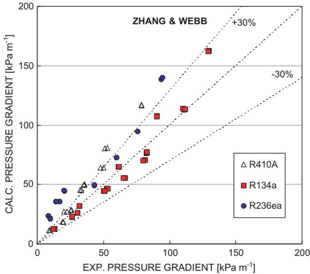
Fig. 17. Calculated vs experimental pressure gradient: the Zhang and Webb correlation.
