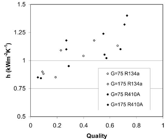
Fig. 8. Condensation heat transfer coefficient data for a 8.91 mm diameter smooth, round tube. Saturation temperature is 35 °C and mass flux (G) is in  $\text{kg m}^{-2} \text{s}^{-1}$ .
