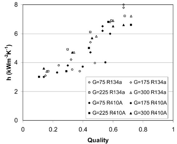
Fig. 10. Condensation heat transfer coefficient data for a 18° helix angle microfin tube flattened to an internal height of 4.15 mm. Saturation temperature is 35 °C and mass flux ( $G$ ) is in  $\text{kg m}^{-2} \text{s}^{-1}$ .
