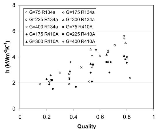
Fig. 11. Condensation heat transfer coefficient data for an axial microfin tube flattened to an internal height of 2.57 mm. Saturation temperature is 35 °C and mass flux ( $G$ ) is in  $\text{kg m}^{-2} \text{s}^{-1}$ .
