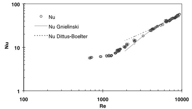
Fig. 4. Nusselt number of the subcooled liquid vs. Reynolds number.
