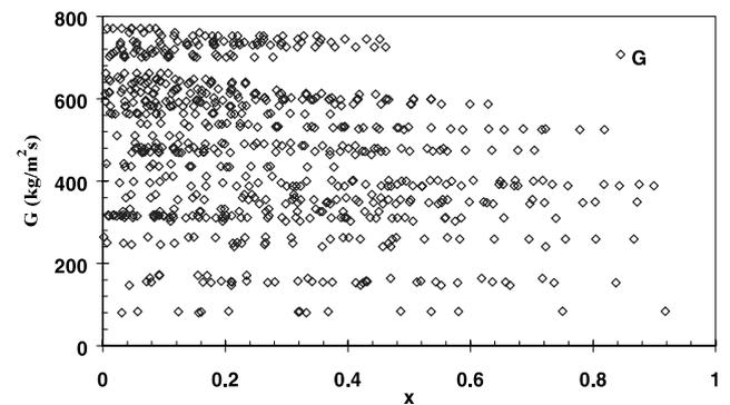
Fig. 5. Mass flux vs. quality for all condensation data points.
