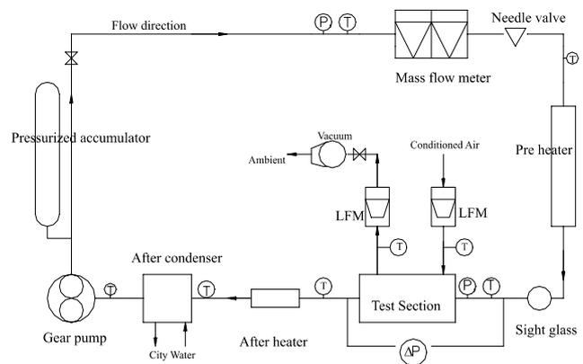
Fig. 1. Schematic of the test facility.
