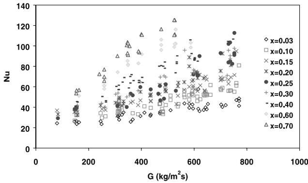
Fig. 6. Condensation Nusselt number vs. mass flux.
