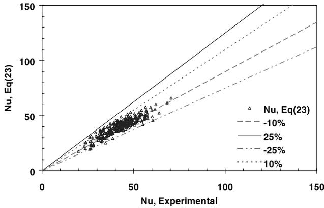
Fig. 13. Comparison of test data with the prediction of Eq. (23).
