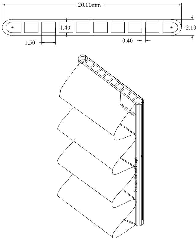
Fig. 2. Condensing test section for heat transfer measurements.
