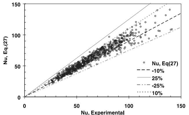
Fig. 16. Comparison of test data with the prediction of Eq. (27).
