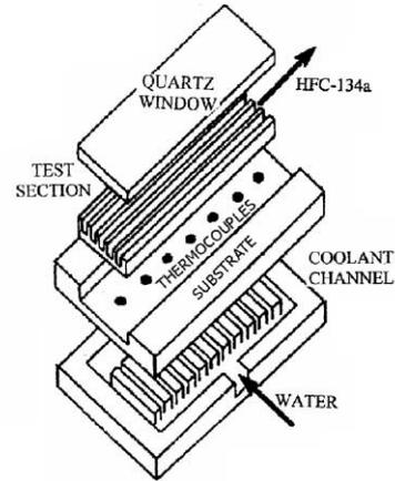
Fig. 3. Condensing test section for flow visualization.
