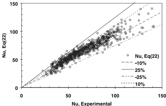
Fig. 12. Comparison of test data with the prediction of Eq. (22).
