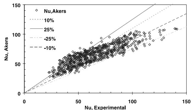
Fig. 8. Comparison of test data with Akers' correlation.
