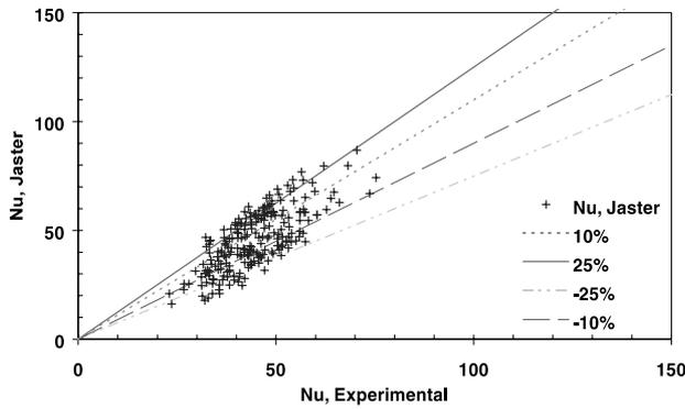
Fig. 9. Comparison of test data with Jaster's correlation.
