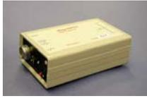
The *Mag-03PSU* provides power to any *Mag-03* sensor via the mains adaptor or the internal rechargeable battery and contains high and low pass filters for the analog signals from the *Mag-03* sensor. The low pass (<4.5kHz) filter removes HF noise from feedthrough of the sensor excitation frequency and any external sources. The high pass (>0.1Hz) filter can be switched to provide ac or dc operation.
