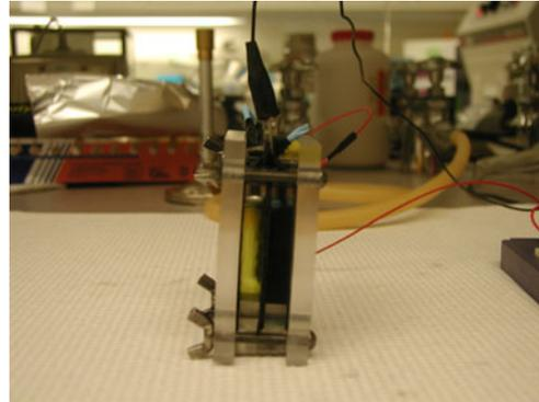
Fig. 4. Leukocyte biofuel cell experimental setup. The apparatus was assembled from parts acquired in a toolkit from the National Center of Biotechnology Education (NCBE).
