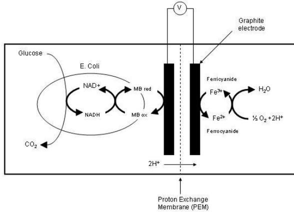
Fig. 1. Illustration of a Microbial Fuel Cell with Methylene blue (MB) as the electron mediator
