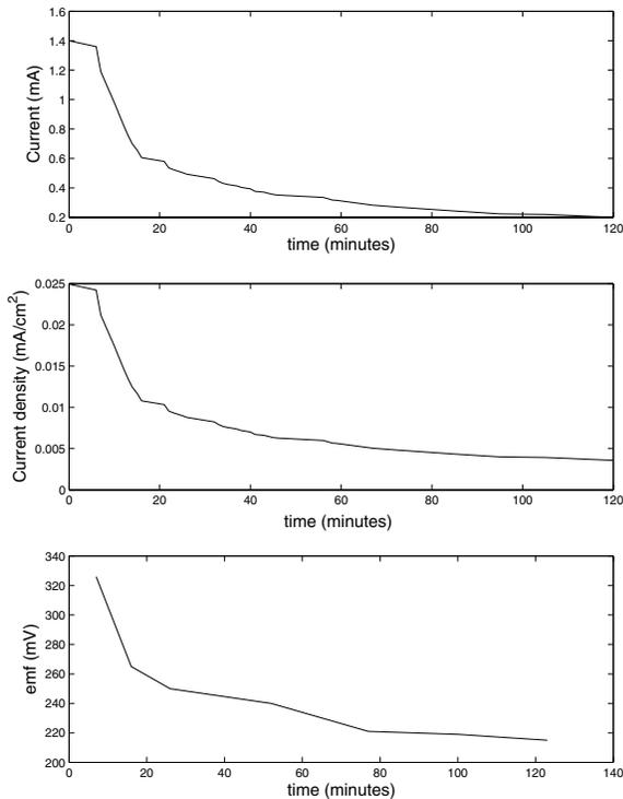
Fig. 3. Measurements of current, current density and electromotive force acquired from the microbial fuel cell
