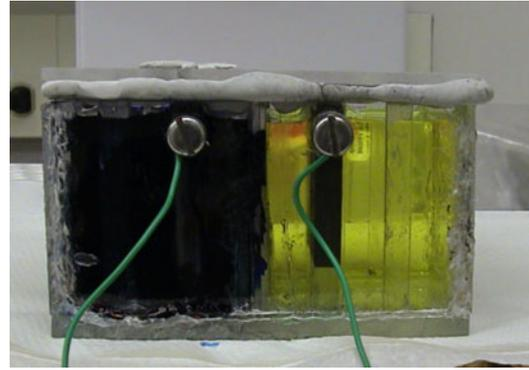
Fig. 2. Biofuel Cell Setup (Front View)
