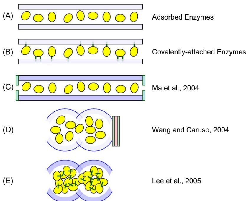
Fig. 3. Several recent advances in the development of stable enzyme systems in mesoporous silica: (A) adsorption; (B) covalent attachment (Wang et al., 2001); (C) partial closure of mesopore inlets (Ma et al., 2004); (D) nanocomposite shell on the particle surface (Wang and Caruso, 2004); and (E) crosslinked enzyme aggregates via a ship-in-a-bottle approach (Lee et al., 2005).
