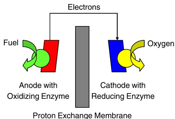
Fig. 1. Schematic of enzyme-based biofuel cells.
