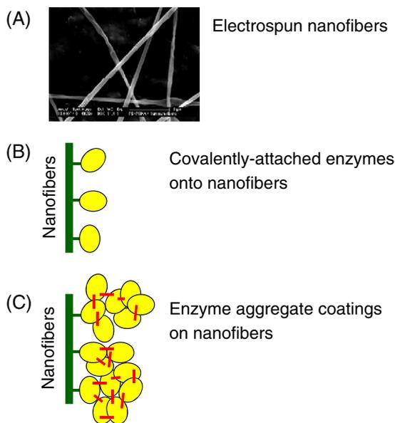
Fig. 4. Enzyme immobilization on electrospun nanofibers: (A) electrospun nanofibers; (B) covalent attachment (Jia et al., 2002); (C) enzyme coatings on nanofibers (Kim, 2005).
