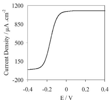
**Fig. 3** Polarization of the 7  $\mu\text{m}$  diameter, 2 cm long glucose electro-oxidizing carbon fiber anode, made with the electrocatalyst formed by crosslinking the electrostatic adduct of glucose oxidase and the “wire” of Fig. 2. Quiescent solution, under air, 37.5  $^{\circ}\text{C}$ , PBS buffer, 15 mM glucose, 1  $\text{mV s}^{-1}$  scan rate.<sup>45</sup>
