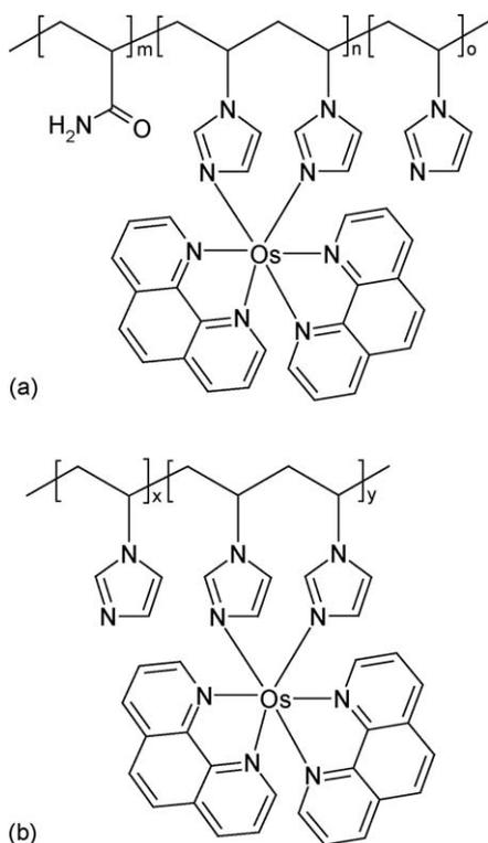
Fig. 1. Proposed structure of polymers IIa and IIb ( $E^{0'} = 0.49$  V vs. Ag/AgCl) designed for the dioxygen reducing cathode, where  $m$  is 17.5,  $n$  is 1,  $o$  is 0.5,  $x$  is 8 and  $y$  is 2, assuming complete reaction of starting material.
