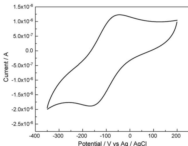
Fig. 4. Cyclic voltammetry of a film of polymer IIIb deposited onto 3 mm diameter glassy carbon electrodes. Scan rate 50 mV/s in 0.05 M phosphate buffer pH 7.4, 25 °C.
