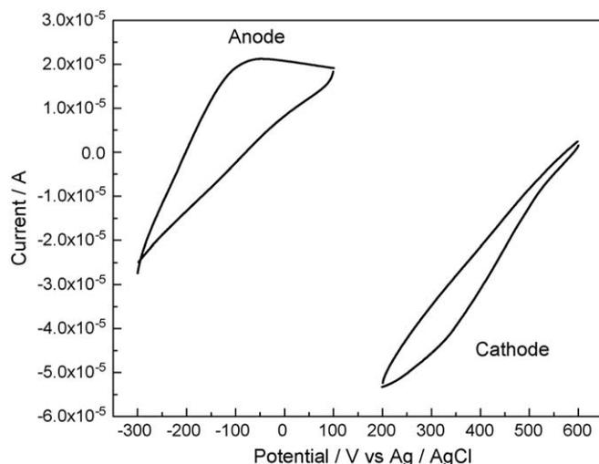
Fig. 5. Cyclic voltammetry at graphite electrodes modified with polymer IIb/laccase (cathode) and polymer IIIb/glucose oxidase (anode) in a single compartment 200 mL cell containing 0.05 M phosphate buffer, pH 4.7, 0.1 M NaCl, 10 mM glucose at 37 °C. Scan rate 1 mV/s.
