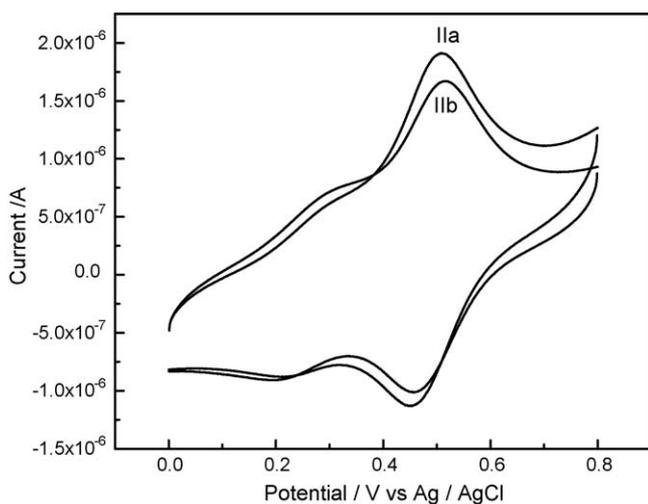
Fig. 2. Cyclic voltammetry of films of polymer IIa and IIb deposited onto 3 mm diameter glassy carbon electrodes. Scan rate 50 mV/s in 0.05 M phosphate buffer pH 7.4, 25 °C.
