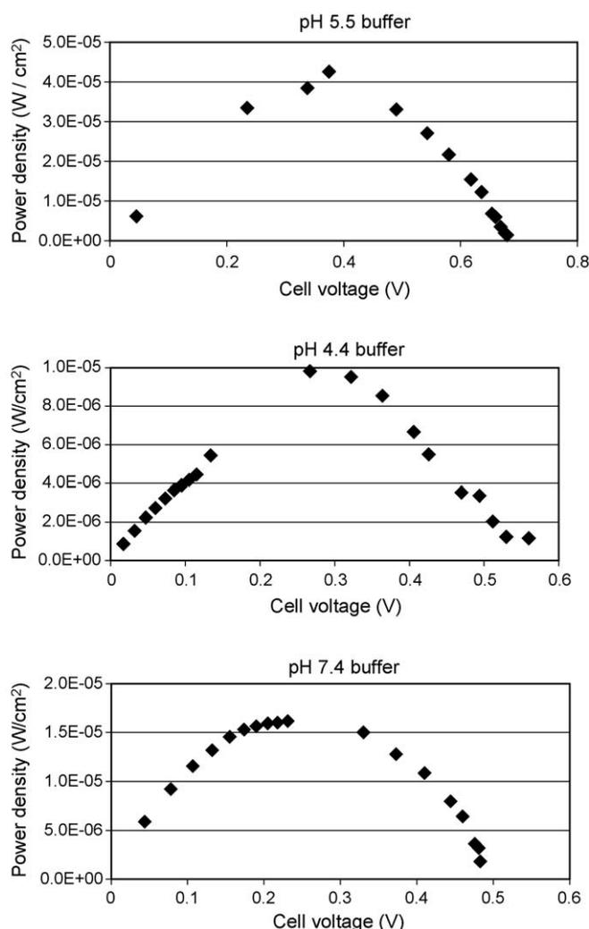
Fig. 7. Power density ( $\text{W}/\text{cm}^2$ ) vs. cell voltage (V) curves at different pH (5.5, 4.4 and 7.4) for a biofuel cell consisting of graphite electrodes modified with polymer IIb/laccase (cathode) and polymer IIIb/glucose oxidase (anode) in a single compartment 200 mL cell containing 0.05 M phosphate buffer, 0.1 M NaCl, 10 mM glucose at  $37^\circ\text{C}$ .
