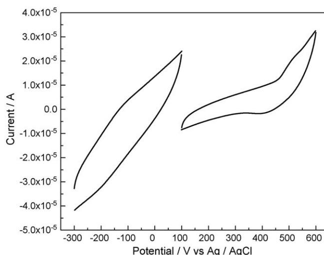
Fig. 6. Cyclic voltammetry at graphite electrodes modified with polymer IIb/laccase (cathode) and polymer IIIb/glucose oxidase (anode) in a single compartment 200 mL cell containing 0.05 M phosphate buffer, pH 7.4, 0.1 M NaCl, 10 mM glucose at 37 °C. Scan rate 1 mV/s.
