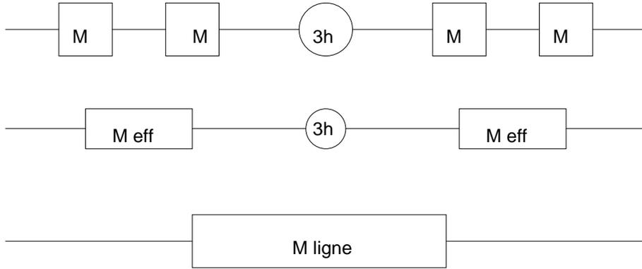
FIG. 7 – Central buffer configuration with  $H = 3h$ .
