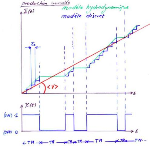
FIG. 1 – Cumulative production for a failure prone production center modeled via an "hydrodynamic" fluid queue picture.
