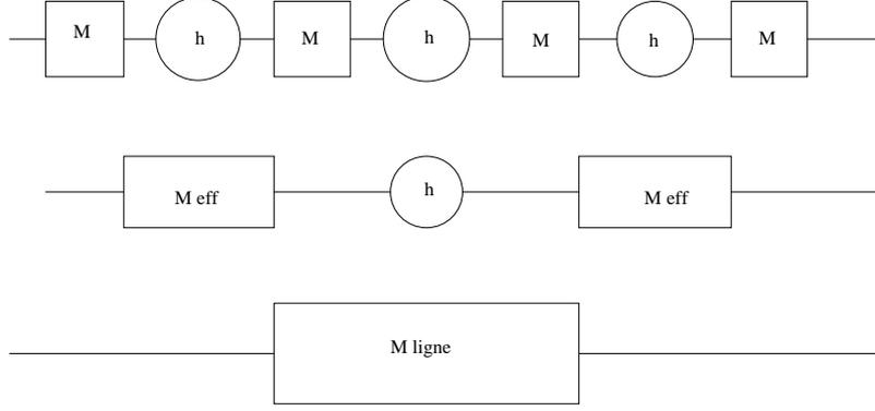
FIG. 8 – Evenly distributed buffer configuration with a total buffer  $H = 3h$ .
