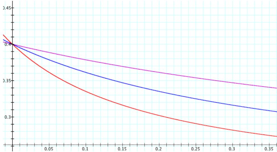
FIG. 4 – Unavailability factor  $\mathcal{J}(h)$  (in ordinate) for balanced  $\mathcal{D}$  with  $\mu = 1$ ,  $\lambda = \mathcal{J} = 0.2$ ,  $\alpha = 1$  (i.e. first line of Eq.(15)) as a function of  $\frac{h}{v}$  (in abscissa) for  $U = 1$  (purple),  $U = 2$  (blue) and  $U = 4$  (red).
